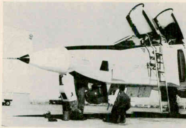
Recording head assemblies and a panoramic-camera reconnaissance system are being mounted in the nose of a supersonic RF-4C reconnaissance aircraft.
