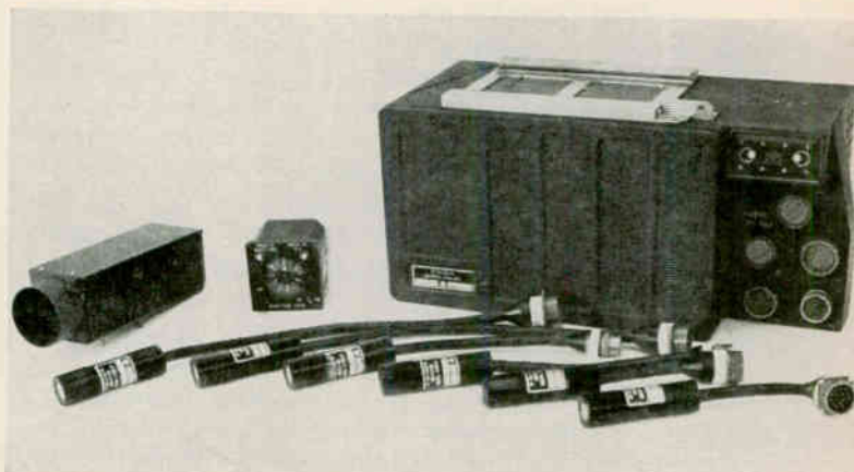
Compact assemblies make up the auxiliary data annotation set (ADAS). The special recording head assemblies are in the foreground; behind them (left to right), is the cockpit test display unit, time insertion unit, and the auxiliary data translator unit.
