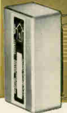
TYPE HGS2MT A medium-sized module, utilizing the extremely fast, highly sensitive HGS mercury-wetted contact switch with minimal contact noise. 2 1/8" long, 3/4" high, 1 3/32" wide.
