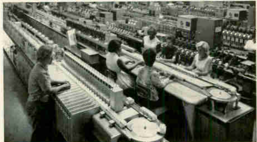
Figure 4. Ultra high speed automatic test machine performs accurate measurements and classifies up to 9000 units per hour
