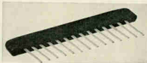
Transistor strings, top, and diode strings, center, are made by bonding chips to package leads. Below is an encapsulated diode string.
