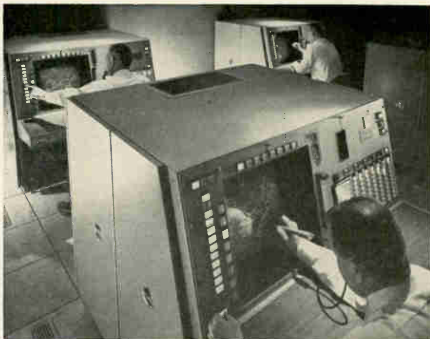
Tv-like consoles show approaching aircraft and the retaliatory forces available. Operators talk with computers by placing a light pen on the aircraft under question.
