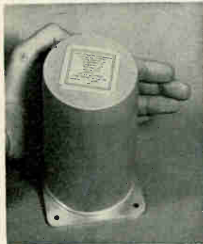
Digital accelerometer is attached to vehicle by four clearance holes on the mounting flange.
