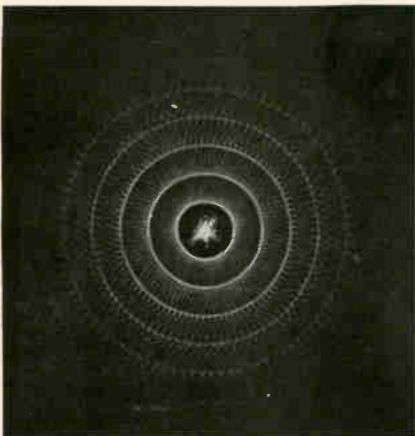
Antenna pattern produced by an array of 96 round antennas set in a ring 1.5 miles in diameter. This pattern, found 2,000 miles out in space, was reproduced in the output focal plane of an optical model a few feet long.
