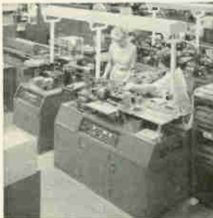
Figure 2. TI's mechanized alloy transistor assembly machine—an industry exclusive—insures uniformity and reliability at very high production rates
