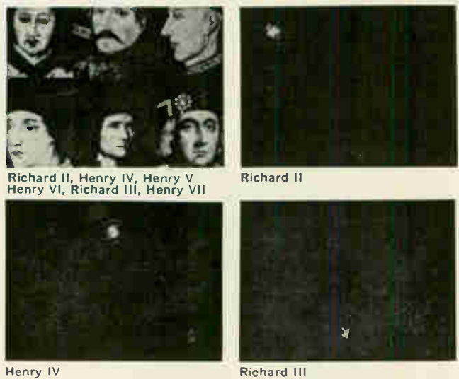
Six English kings identified by optical matched filtering. A filter corresponding to each face identifies that face in the presence of noise (other faces), and produces a bright spot on the output plane.
