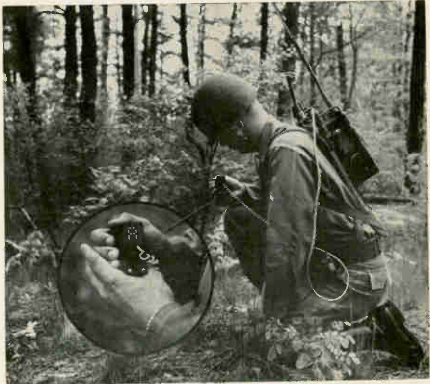
Morse code converter translates dot-dash-dot into letters.
