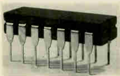
The original dual in-line package, made by Fairchild Semiconductor.
