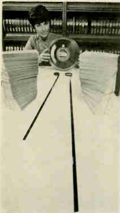
Strips of magnetic computer tape contain equal number of digital bits. Data on shorter tape is encoded with IBM's new phase technique, which doubles digit density.
