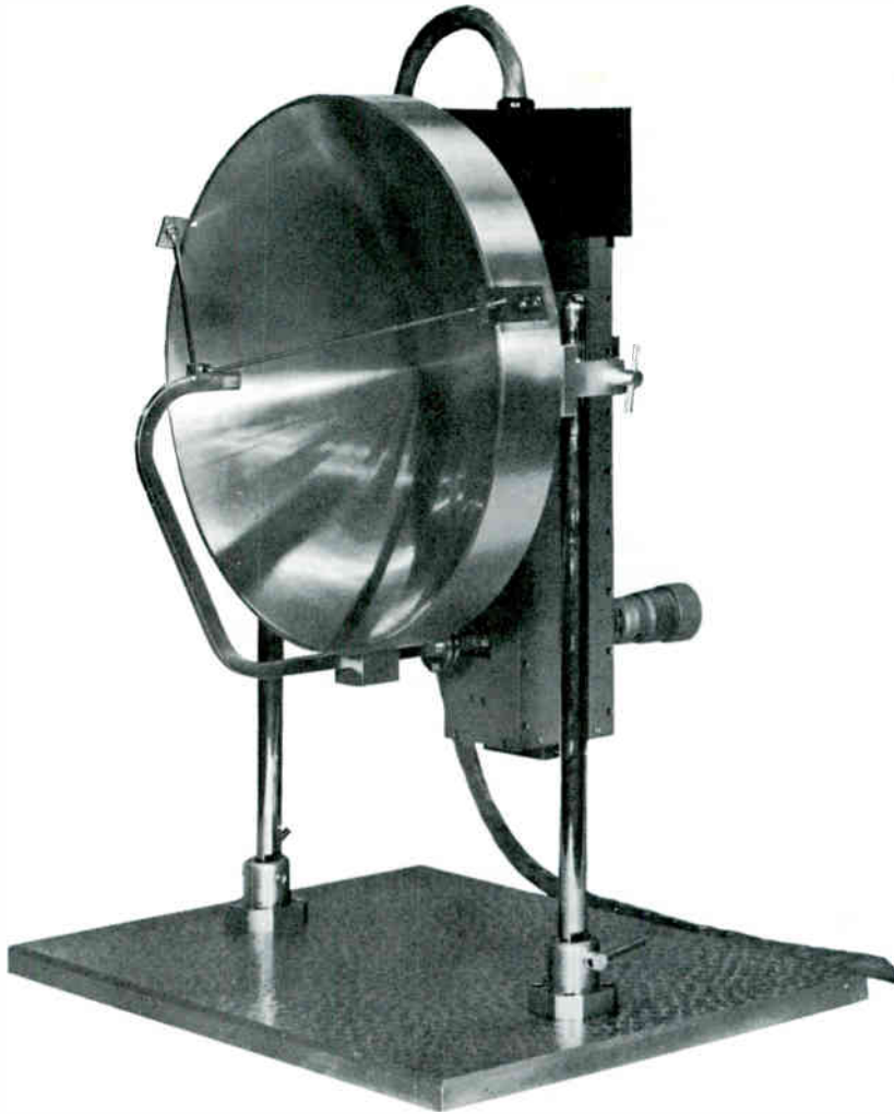
Elliptical antenna focuses microwave energy to a point 17 inches away. It is used for measurements on targets that are relatively inaccessible. Heat sink, at top of assembly at rear of antenna, dissipates heat from klystron.
