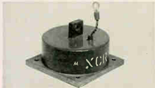
Array of scr's is shown with resistors attached to cathode leads of individual rectifiers. The entire unit is covered by a metal case.
