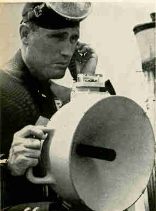
Berry L. Cannon uses the AN/PQS-1B sonar to search the ocean floor.
