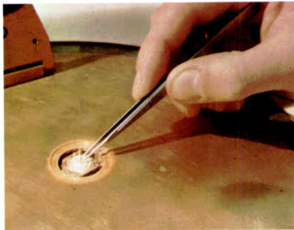
Pellet-mounting process. Here, the header is being inserted into a heating chamber. After a 30-second warm-up period, the pellet is placed on the header and connected to it with a gold-silicon alloy.
