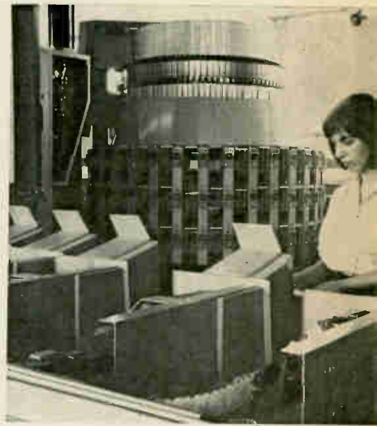
Mail sorting is masterminded from central electronic rack at left, which provides memory and logic. Girl at right stamps zip-code destinations on envelopes, which are sorted in the chandelier-like tower to her right.
