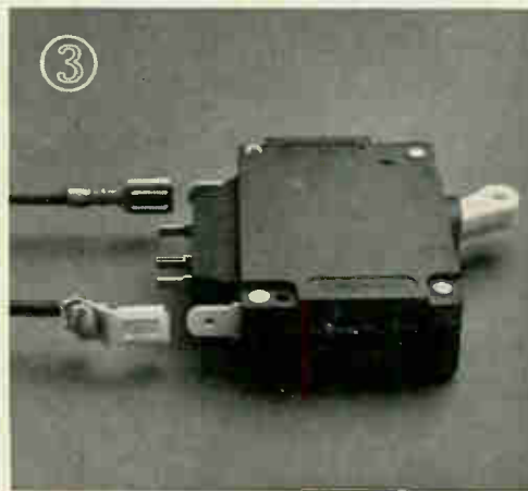
Aquasonics communicator is a 42-Kc a-m, device with 1,000 foot range
