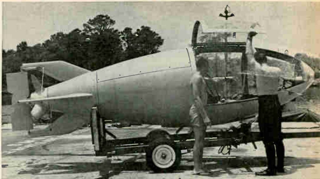
Wet submarines travel at 9 knots but are too maneuverable to use at deep levels where a quick ascent would be dangerous to aquanauts. The miniature sub might be used by surface divers to take supplies to Sealab.
