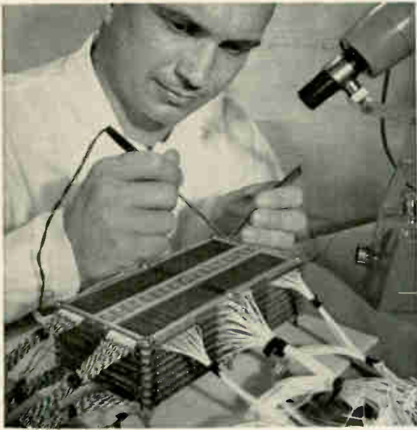
Memory stack (above) can be repaired by using spare words in each plane. Stack is built by wiring board edges (right) and folding up the planes.
