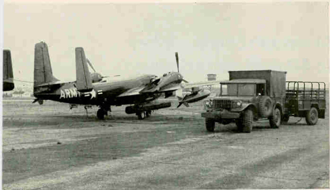
A truck containing the Mohawk adapter test unit (AN/ASM-88) drives up to an Army OV-1B to check its radar. No connection to the receiver or transmitter is necessary.
