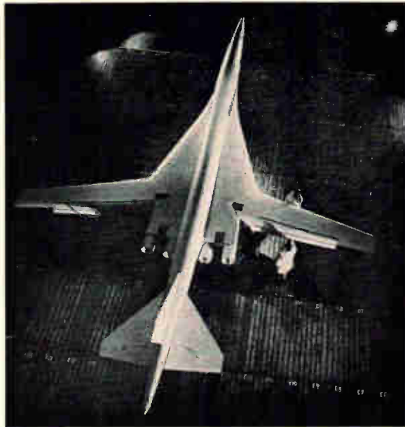
One model of supersonic airliner being prepared for wind tunnel tests at Boeing Co.
