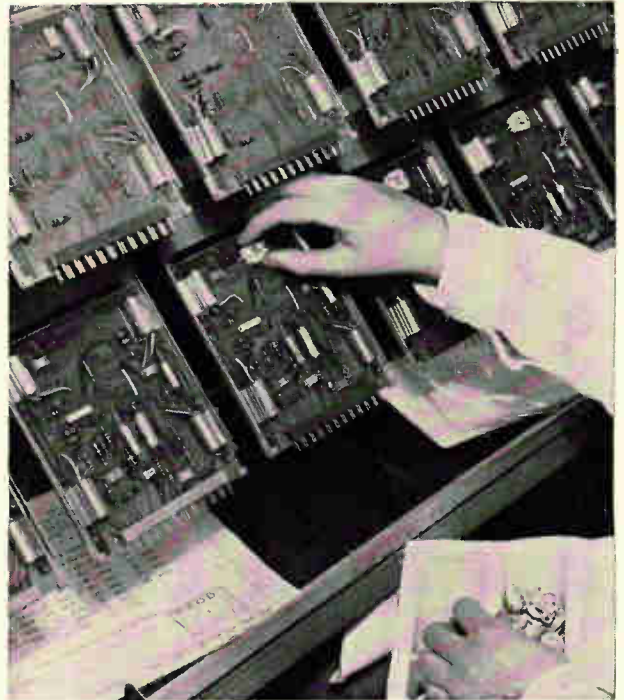
Partially assembled cards, awaiting delivery of parts, can get free ride on top deck while assembly proceeds below.
