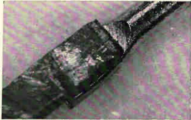
Kovar lead of flatpack is lap welded to nickel wire.
