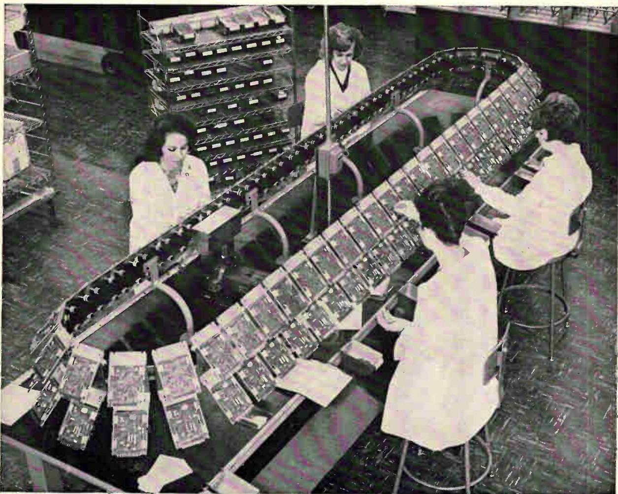
Double-decker line allows operators to work on two production runs simultaneously, or to divide tasks on one run for higher production rate.
