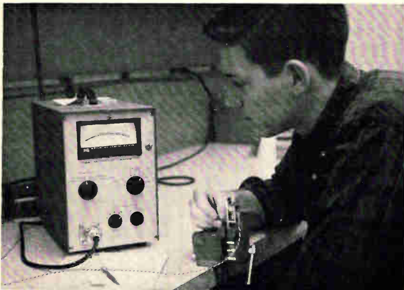
Testing the accelerator in the laboratory with simulated application of stress caused by acceleration. Several accelerators were built to monitor changes in acceleration to 100 g's. The accelerators were designed to operate with 28-volt battery supplies. Typical variations in output signal caused by changes in stress sometimes exceeded one volt.
