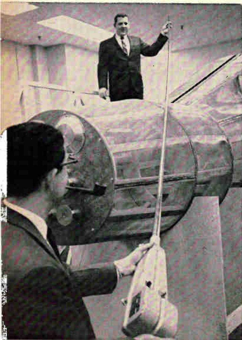
Fully extended, the h-f voice antenna is 13 feet long. In background is full-scale wire mockup of spacecraft, which is used to measure antenna impedance and voltage standing wave ratio.
