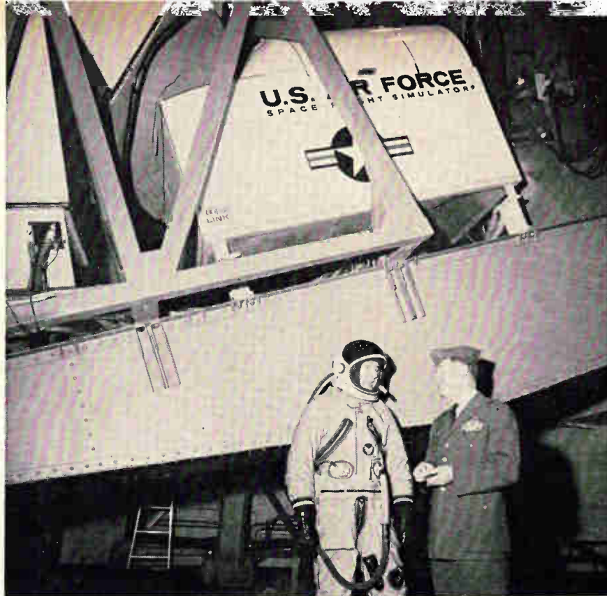
Prodan and school commandant Col. C.E. Yeager chat while waiting for the spacecraft to be brought into boarding position. The 15-ton mechanism makes the cockpit vibrate like the Titan II.
