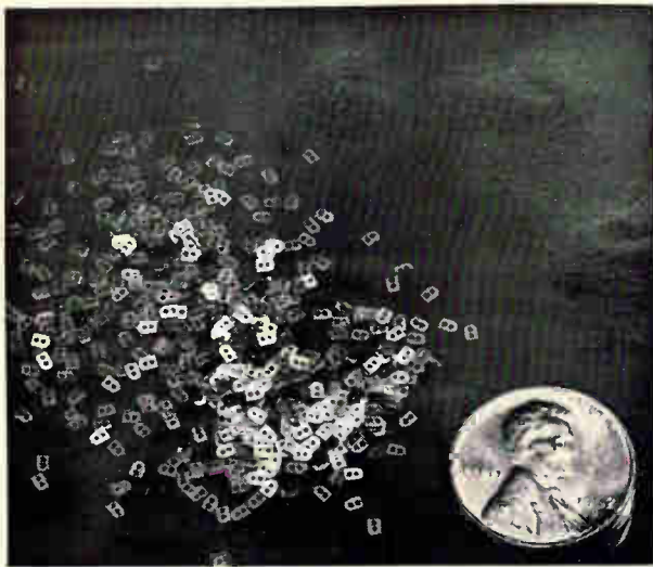
Ferrite memory cores used in the Gemini computer measure less than one-tenth of an inch in length. There are over 150,000 of them in the computer.
