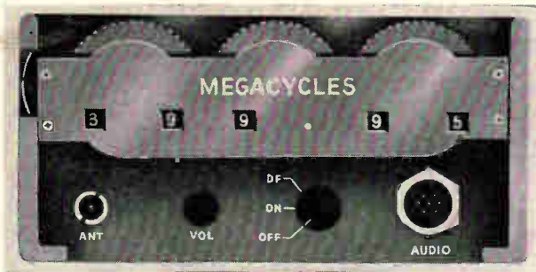
Digital switches like that of the AN/PRC-66, shown above, will set up transmit/receive frequencies in less than 5 seconds.
