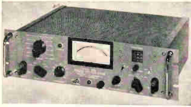
Vector voltmeter can measure in-phase and quadrature components of voltage while rejecting noise and harmonics over the entire frequency range.
