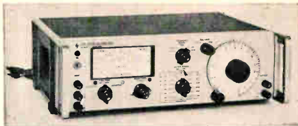
Model 331A distortion analyzer can be bench- or rack-mounted. Controls are simple to use; meter, calibrated in decibels, percentage and volts, is easy to read. The frequency, set with the large dial, is accurate to within 2%.
