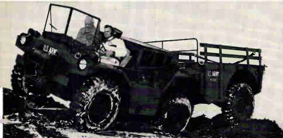
PATA crosses hard and soft terrain on continuous track of air-filled cells.
