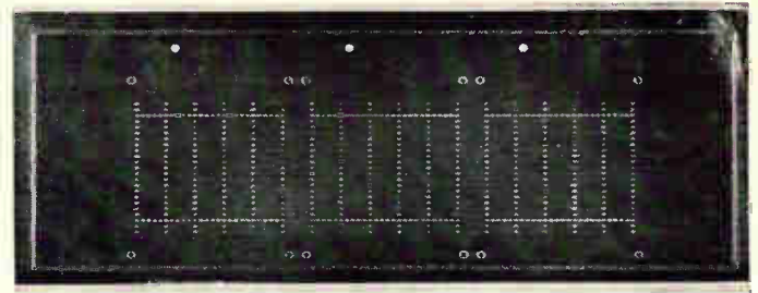
Plated riser laminate with three riser patterns. The risers are prefabricated feedthroughs and weld pins.
