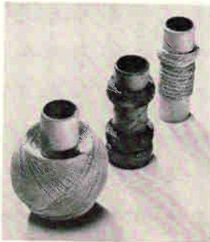
Machine can be used to wind coils into unusual shapes.
