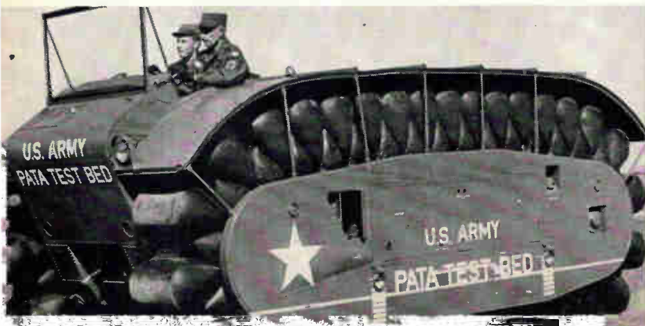
PATA crosses hard and soft terrain on continuous track of air-filled cells.
