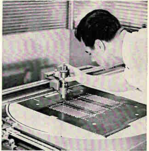
Worst-case test pattern for etched circuit is scribed on a coordinate drafting machine. Note registration-hole pattern around edge of circuit pattern.
