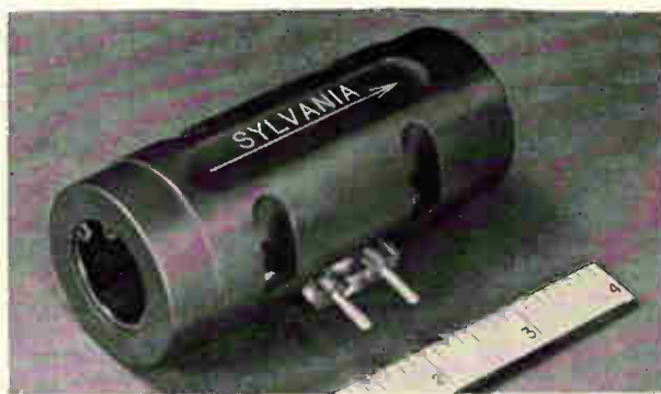
Coherent-light optical modulator is inserted between laser beam source and output of the laser transmitter. Modulation is usually limited to 30%, requiring an applied voltage of 110 volts.
