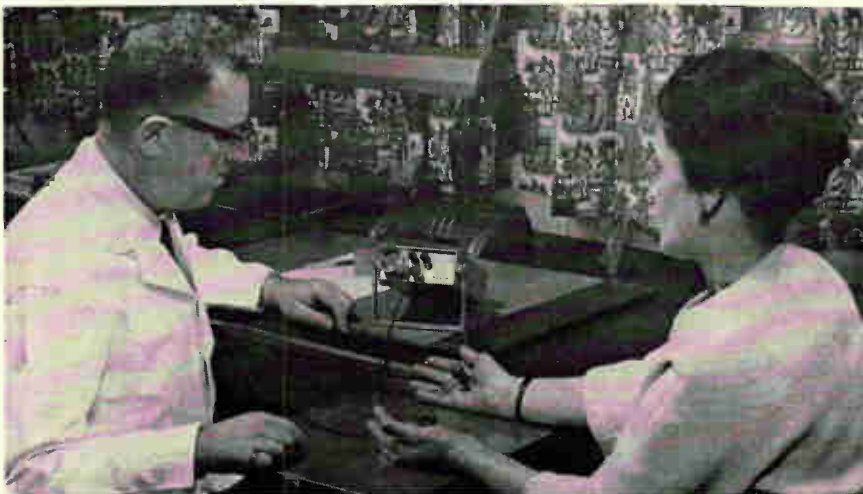
Electrocardiogram is taken with the new Miniscope. Portable instrument from Westinghouse Electric Corp. provides clinical data on patient's heart.
