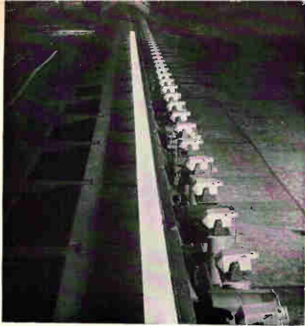
Hot billets are sized as they whiz past 72 infrared-sensitive photocells. Data goes to billet-cutting computer.
