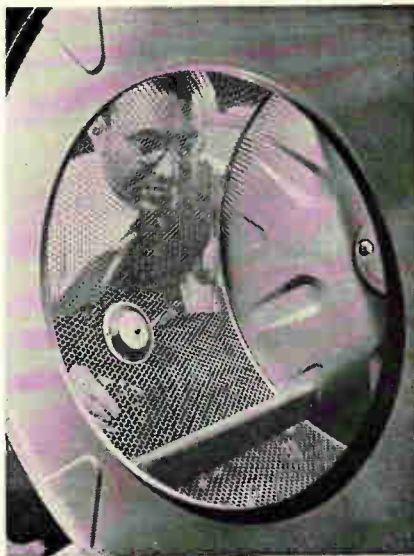
Button senses moisture of laundry in home clothes drier. When the laundry is dry, circuit turns off drier.
