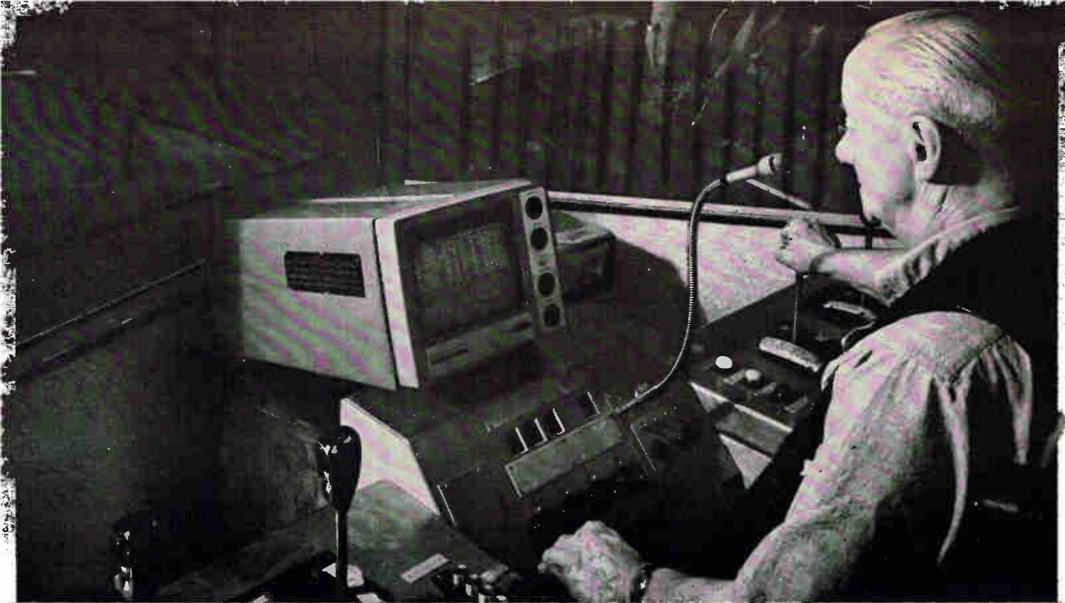
Operator controls cutting of blooms after reading computer-generated instructions on the face of the cathode-ray tube display.
