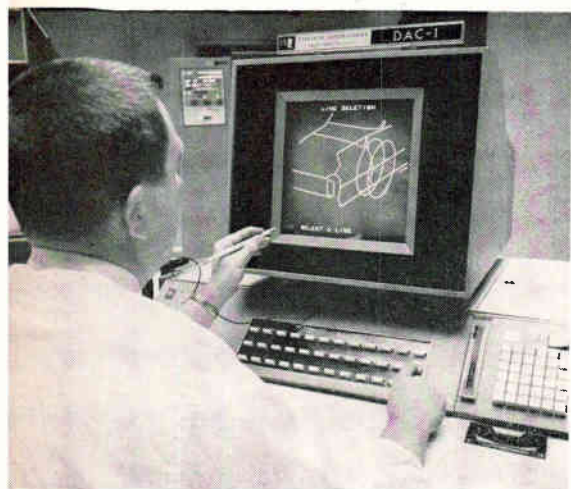
Electronic styling lets designer at GM add or remove a line by pressing the proper button and running a light-pencil over the face of the display. He can also enlarge a view or change the perspective.
