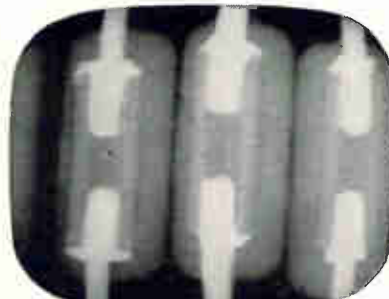
Glass resistors with holes, cracks
