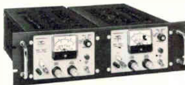
Two Trygon HR20-1.5's, rack-mounted side by side.
