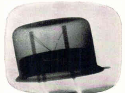
Transistor with broken lead
