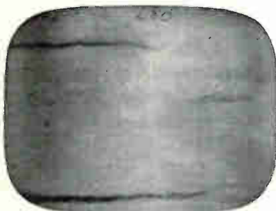
Cracks in a titanium weld
