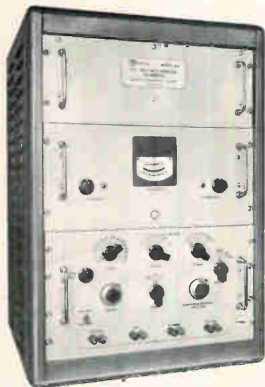
Model 64 DC Voltage Calibrator — gives simple, rapid and accurate DC instrument calibration. Automatically divides range into as many as 15,000 equal parts. Accuracy within \pm 0.05\% of indicated value.
