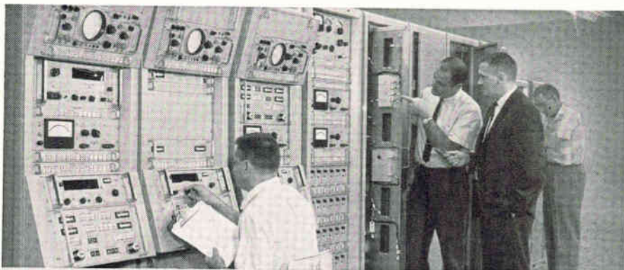
A Motorola RF Receiver Subsystem for DSIF will Provide Communication Links Between Earth and Vehicles on Future Interplanetary Flights.
