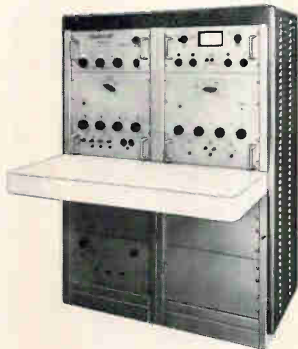
Model 172 Variable Frequency Calibration Console—provides current and voltage output within \pm 0.05\% of reading, up to 2500 cps. Wattage outputs within \pm 0.1\% . Variable frequency output from 50 to 10,000 cps. Short term stability 0.01%.
