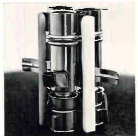
After being cleaned in quick-drying FREON TF, the residue-free subassembly is ready immediately for final processing.
