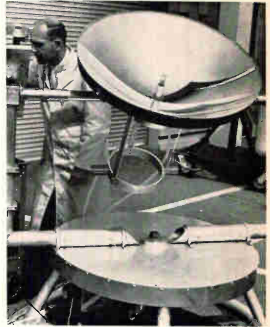
Parabolic mirror concentrates sun to pump laser.
