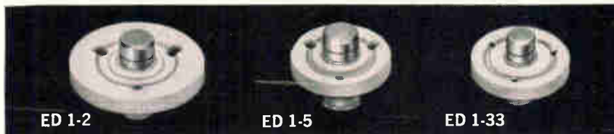
Standard ED 1-2. (.121" OD shank, .490" ceramic). Most widely used cathode. Standard length, .312".
