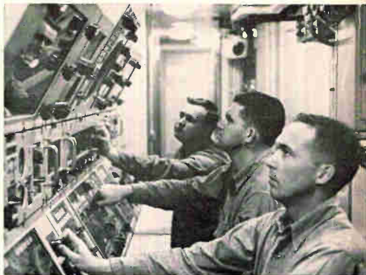
Attack center in control room. There are two complete fire-control panels. Each accepts range and bearing data from sonar, radar or visual sightings. For training purposes, one panel can furnish simulated targets to the other panel.
