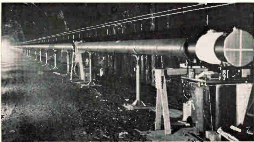
Mockup of linear accelerator housed in an abandoned railroad tunnel. A gas laser will provide a light source for optical alignment in the 10,000-foot-long accelerator.
