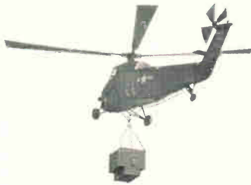
24-channel, dual-diversity, 1 kw tactical tropo terminal in S-144 shelter—total weight only 1500 lbs.
