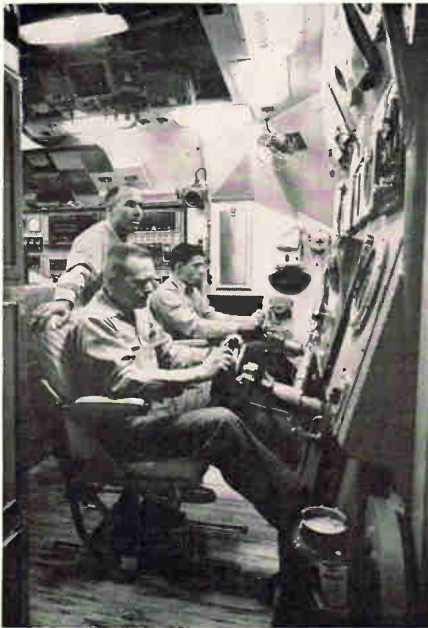
Control center of submarine. Sailor in foreground is helmsman or inboard planesman. He controls course, speed and angle of sail planes. Beside him sits the outboard planesman who controls the angle of the stern or main diving planes. The diving officer stands behind the planesman. Panel in background is ballast control, diving station of the Chief of the Watch.
