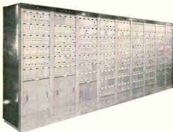
Half the space and three times the control are offered by the servo system, bottom photo. Its predecessor, the tube version, top photo, was the normal setup until transistors were introduced.
