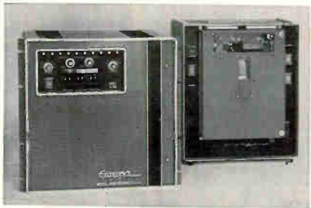
Portable data processor by Epsco Inc., Cambridge, Mass., has been used to field-test automotive components. Up to 100 sensors measure shock, vibration, acceleration and other variables while the car is in motion. Signals are digitized to 1 part in 1,000 at 20,000 samples per second.
