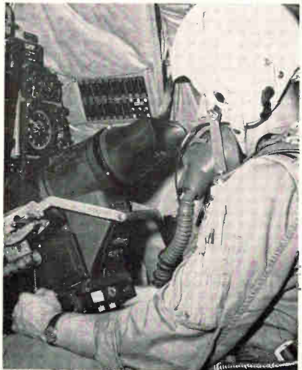
Navigator—also on the EMR team. This navigational radar scope helps establish the position of the Air Force RB-66C Destroyer in the air. Above the scope is an N-1 aircraft compass and above the compass are a dial and a clock.
