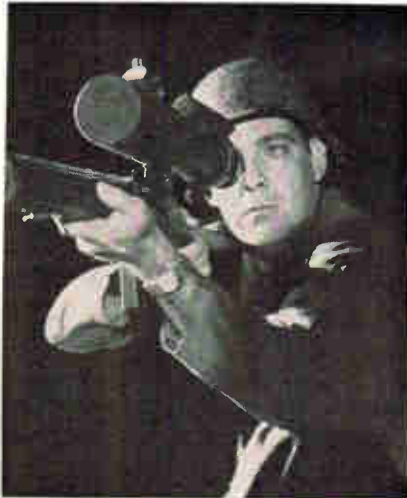
Army weapons sight using cascaded image-intensifier tubes will be in the hands of troops next year. It intensifies low-level light 80,000 times.
