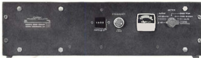
NEW Type 1115-B Standard-Frequency Oscillator . . . $2050 A 5-Mc, 5th-overtone crystal oscillator with a short-term stability of better than 1 \times 10^{-11} , measured over a 1-second averaging time . . . additional outputs at 1 Mc and 100 kc . . . all silicon transistor circuits . . . built-in battery supply and charger for emergency operation up to 35 hours . . . spectral line width less than 0.25c at 10 Gc.
