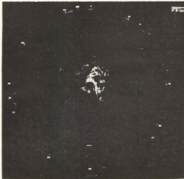
Typical PPI presentation of a radar video signal in heavy clutter. Target at 180° is lost in the weather return.
