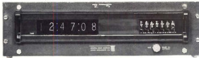
NEW Type 1123-A Digital Synchronometer® Time Comparator . . . $2950 A solid-state digital clock for time and frequency standardization . . . operates with the 1115-B Standard-Frequency Oscillator for time comparisons to 10 \mu sec . . . Numerik in-line readout of hours, minutes, and seconds . . . readout can be programmed to read up to 100 hours before recycling. Self-contained 24-hour emergency power supply.
