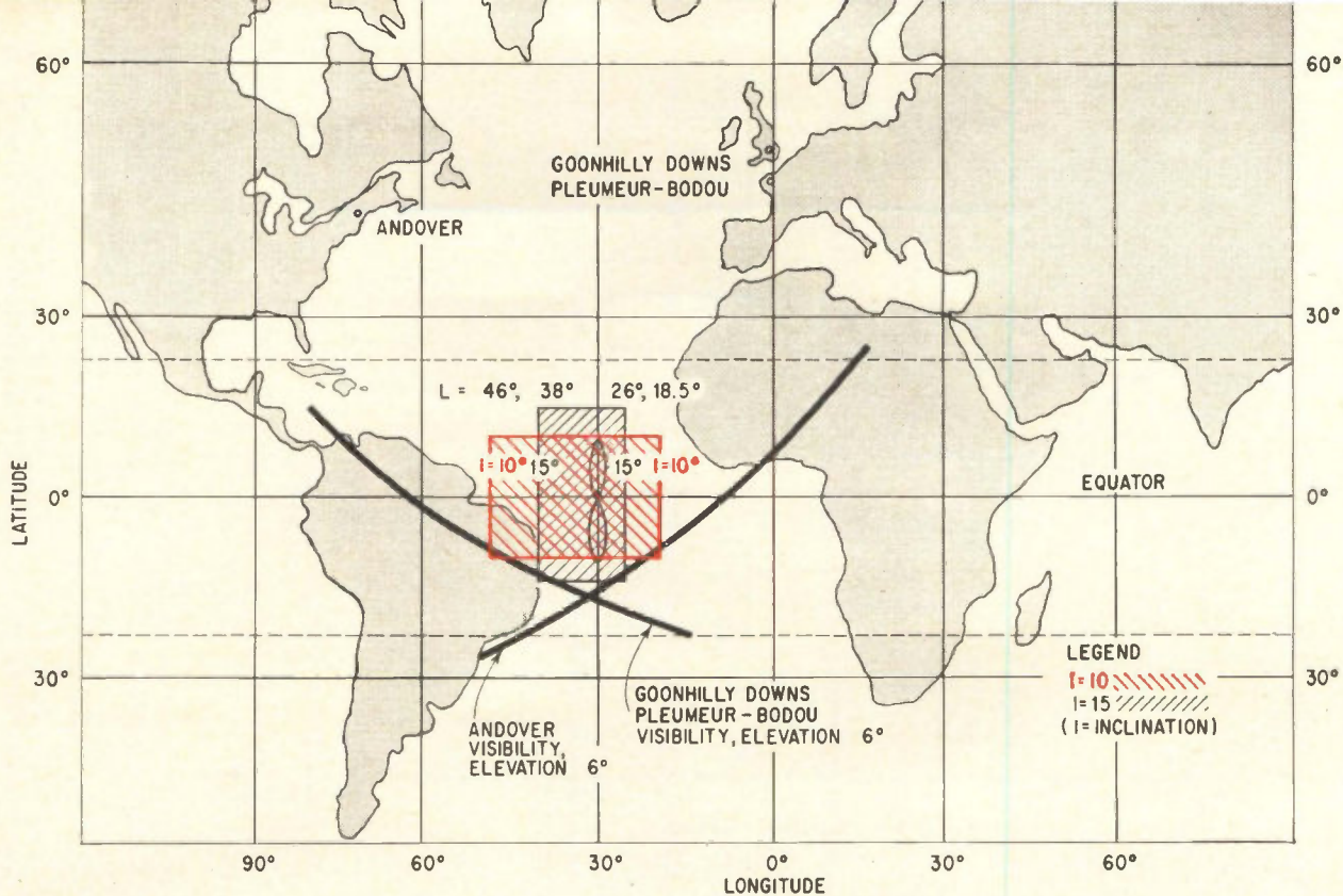
Visibility limits for 10 degree and 15 degree inclined synchronous orbits of the HS 303.
