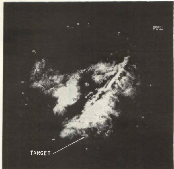
Typical PPI presentation of a radar video signal in heavy clutter. Target at 180° is lost in the weather return.
