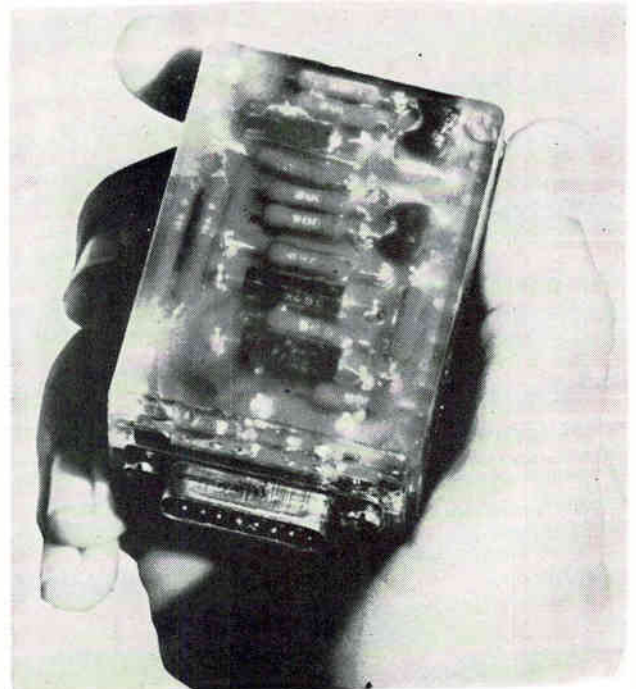
OSCILLATOR used in telemetry system of the Q-2C jet target drone employed by Navy and Air Force for testing ground-air and air-to-air missiles. Designed to withstand 25 water landings and recoveries, the unit has been encapsulated in a room temperature vulcanizing clear silicone elastomer supplied to the manufacturer, Dorsett Electronics, by General Electric. Besides absorbing vibration energy, the silicones serve as short-term high temperature, insulators. Components can be cut out and replaced
