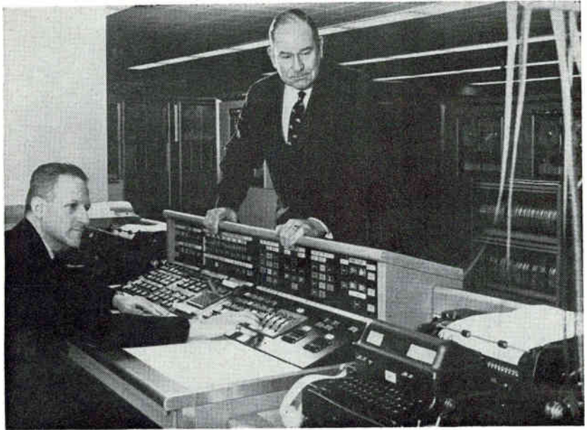
TEST RUN on RCA Communications new switching center in New York where computer devices speed up teleprinter message handling and provide billing data. R. K. Andres demonstrates the command and interrogation features while president T. H. Mitchell looks on
