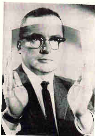
LIGHT-SENSITIVITY can be confined to one part of the glass, as shown. The upper area lets through about 30 percent of the visible light. The lower part allows 86 percent light transmission
