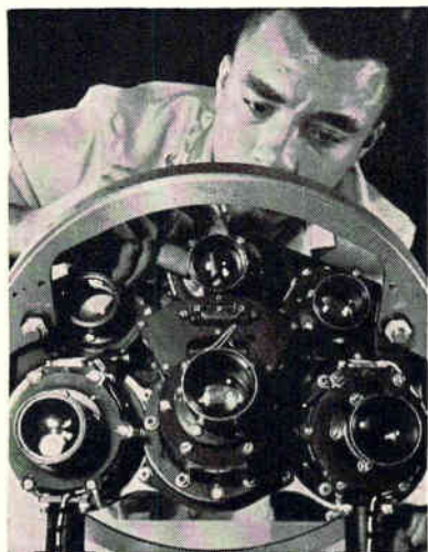
SIX TV CAMERAS —three wide-angle and three narrow-angle—will take the first close-up tv pictures of the moon
