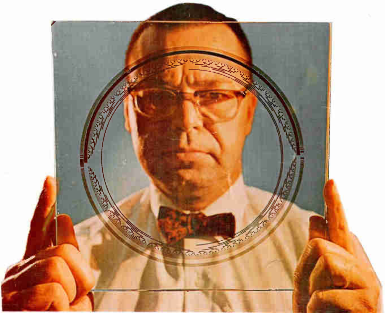
DISK ENCODER is photographically produced using a diamond-ruled master die.
