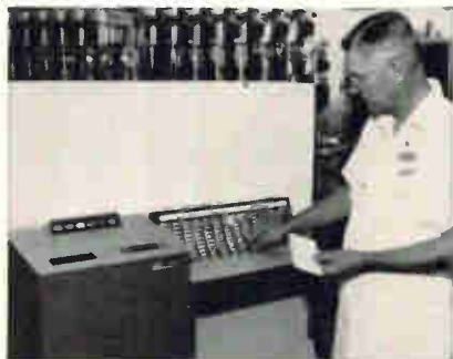
The IBM 357 Data Collection System records information, from any location in your plant, directly onto IBM punched cards. Input stations record data from badges, cards or manual keyboard.
