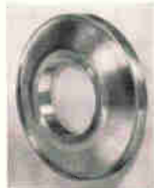
OFHC COPPER (Ring Forging, Rough Mochined)
