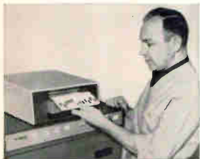
IBM 1030 Data Collection Units are installed anywhere you need them throughout your factory. Employee uses new IBM data cartridge to record information and transmit it to the central computer.
