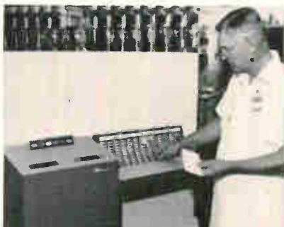
The IBM 357 Data Collection System records information, from any location in your plant, directly onto IBM punched cards. Input stations record data from badges, cards or manual keyboard.
