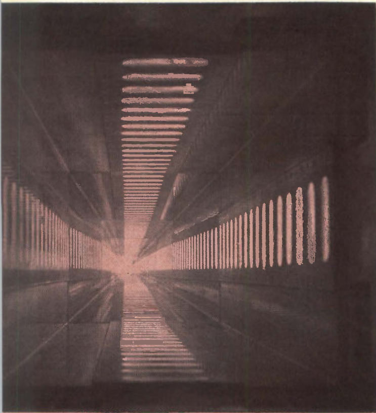
WAVEGUIDE antenna feed is 96 ft long with below-resonant, series, transverse slots spaced about 0.2 wavelength apart. Normally operated with circular polarization, the feed can also use linear polarization resulting from in-phase excitation of corresponding orthogonal slots
