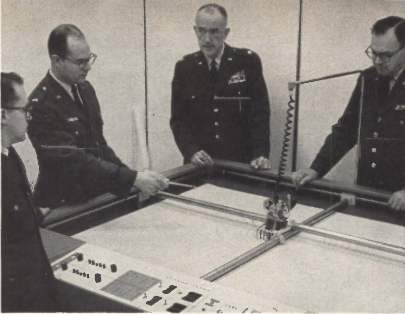
PLOTTER tied into 7030 gives target and trajectory data pictorially
