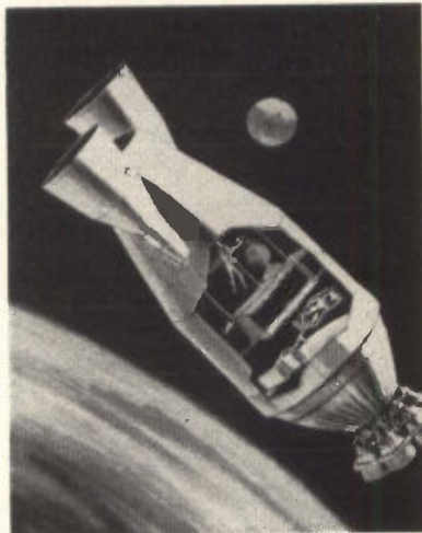
GEMINI CAPSULES attached to station conceived by Douglas. Cutaway shows whirling centrifuge couch that creates artificial gravity
