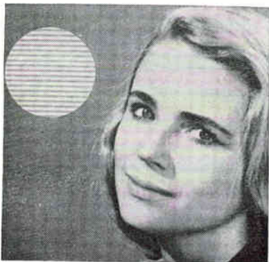
TELEVISION film recording made on 16-mm film by direct electron exposure. Lines are clearly resolved as shown in inset, top left
