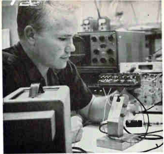
L-BAND offset doppler (ODOP) phase-locked transponder for Saturn is checked out at Motorola. Receiver threshold sensitivity is -130 dbm; transmitter power output is 1 w min
