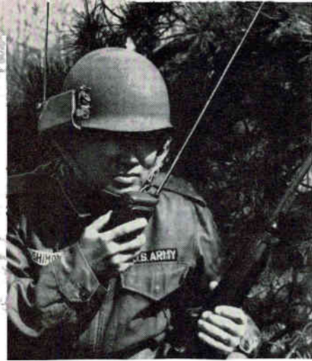
HELMET-ATTACHED receiver and hand-carried transmitter are expected to improve combat control
