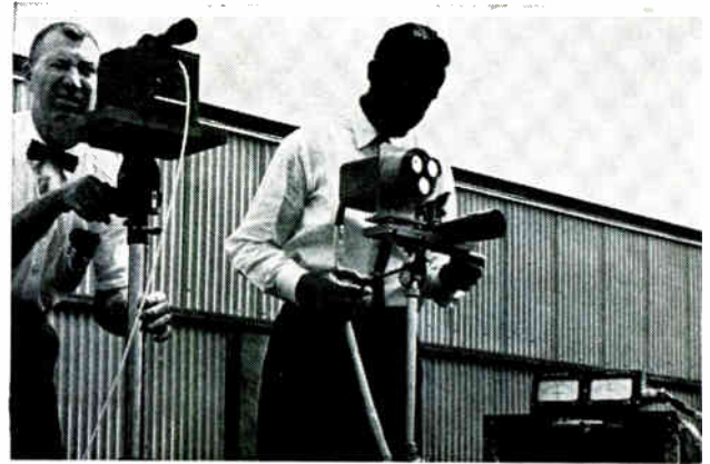
EXPERIMENTAL transmitter (left) and receiver (right) are manually aimed. Servo coupling would make operation automatic
