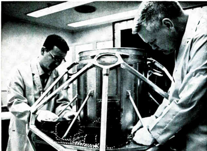
SANDIA LAB personnel install logic system in Vela Hotel satellite frame. X-ray detectors go into holes in triangular points of frame
