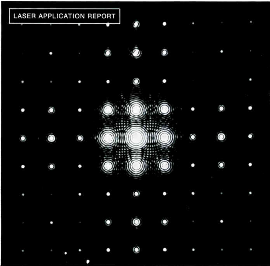
Far-field diffraction pattern produced from laboratory model using coherent light.
