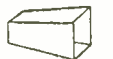
4. OPEN END FORMER... forms open end shapes by replacing box fingers with open end finger.
