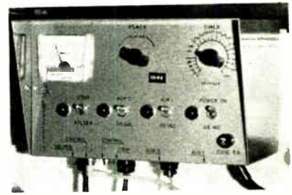
SOLID STATE supply provides adjustable current pulses to probe. A foot switch controls the supply but machine turns off at a predetermined time
