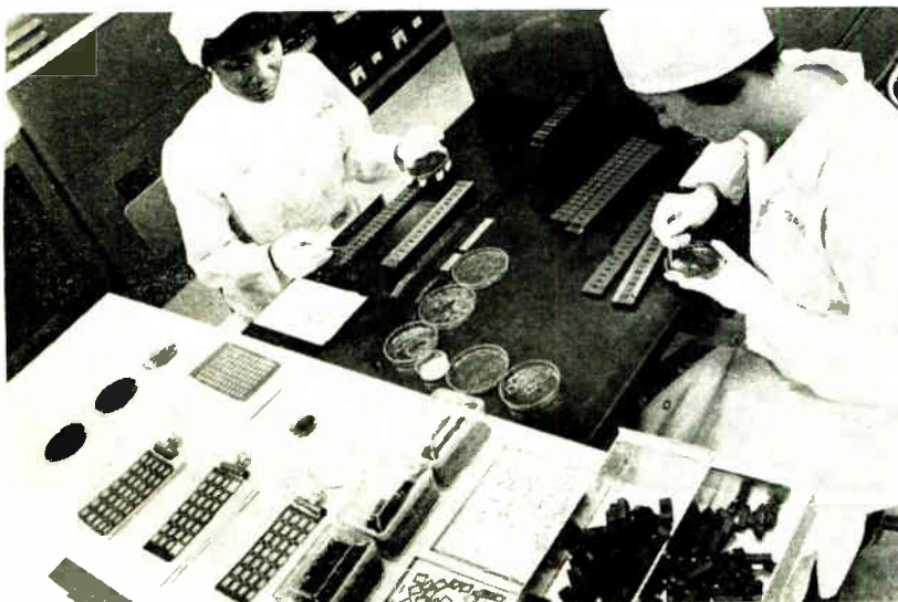
FINAL ASSEMBLY and packaging of integrated circuits manufactured by the Westinghouse Molecular Electronics Division, Elkridge, Md.: The Kovar alloy frames in the petri dishes are placed in the carbon casts on the workbench. Glass, Kovar alloy leads, and metallic or ceramic bases are then added. Weights from the boxes at lower right are placed on top. The entire assembly is fed into the inert gas furnace, top right, where the glass fuses to form an hermetic seal. Called Flat-Packs these circuits are functional blocks.
