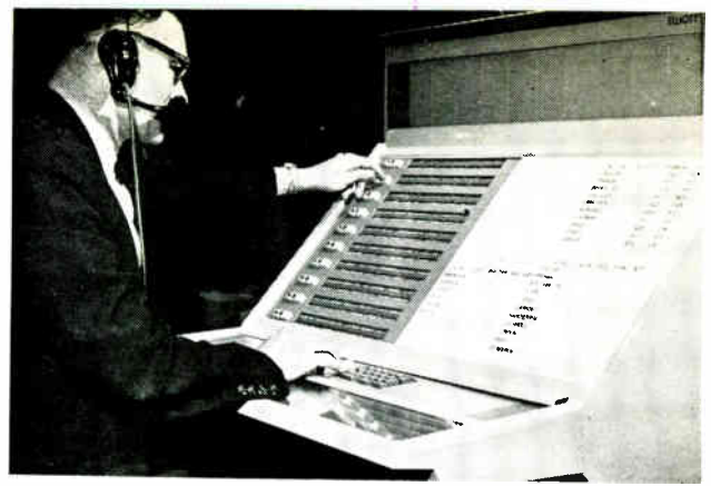
ALPHANUMERIC indicator driven by Elliott 502 computer updates airport controller's information
