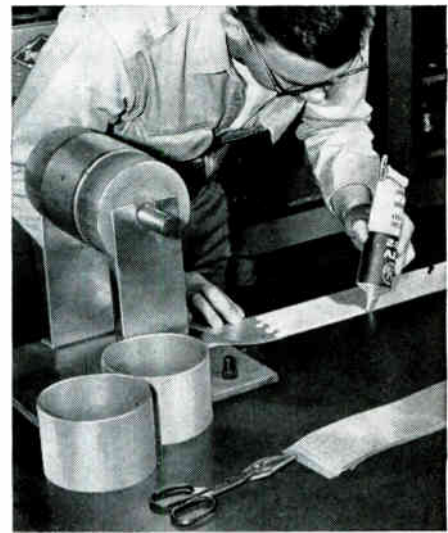
Manufacture it. RTV adhesive/sealants are fast working assembly tools, eliminate prefabricated parts or more costly, time consuming techniques. Here an RTV adhesive laminates flexible mica strips to form cylindrical ducts.
