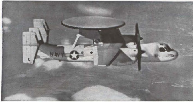
BIG ROTODOME gives E-2A Airborne Tactical Data System aircraft distinctive look. Plane carries 5-man crew. Grumman is prime contractor for the system
