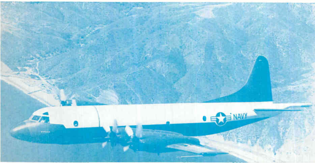
ASW PATROL PLANE, Orion, helped Navy track and flush Soviet submarines during the Cuban crisis. Extending from tail is magnetic anomaly detector
