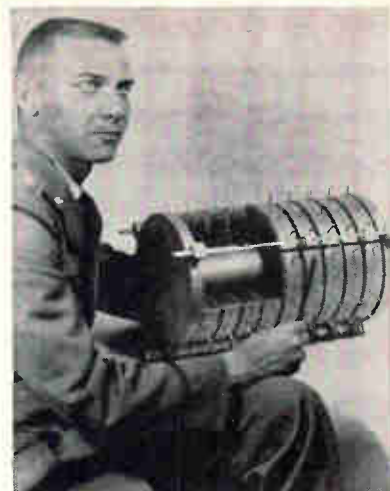
FOOT IN DIAMETER and three feet long, "atomic heat engine" will convert a small reactor's atomic heat directly to electricity, operating in a manner analogous to thermionic diodes. The power converter shown here is a half-size mockup
