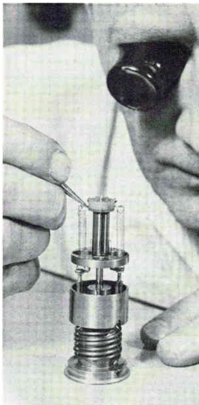
AXIAL accelerometer is assembled prior to test at radiation levels of 1.5 \times 10^{16} fast neutrons/cm 2 (Giannini)
