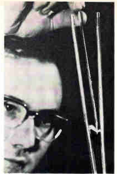
BORON nitride takes 10,000 volts. Strip is 1/32-in. thick
