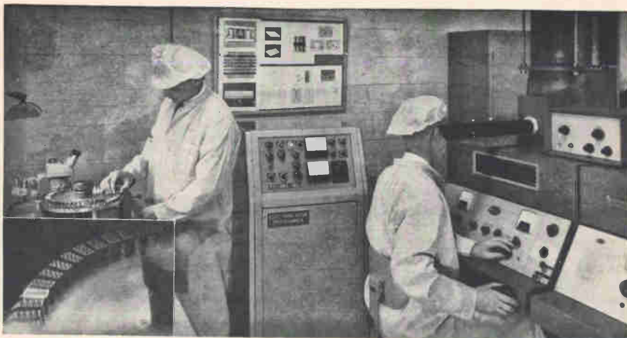
POSITIONING FIXTURE is loaded with relays during welding of other relays. Inset shows multi-exposure photo of beam-impingement traverse on relay. Beam travel is controlled by specially-designed programmer unit in center
