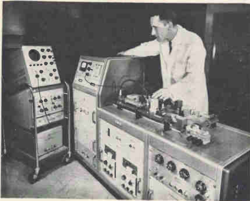
EXPERIMENTAL waveguide system for telemetering 3,000 channels from space vehicle in space-environment test chamber is demonstrated by feasibility model, above. Diagonal unit at right is model of waveguide network
