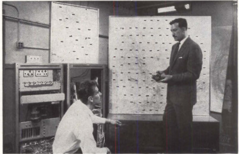
COMPLETE SYSTEM including a subsidiary display at upper left. Photo code wheel is in control unit; author Collis is standing—Fig. 1
