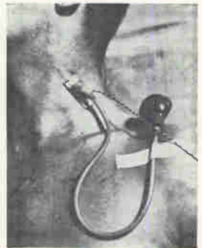
PIEZOELECTRIC ultrasonic transducer for monitoring changes in blood flow, from the University of Washington
