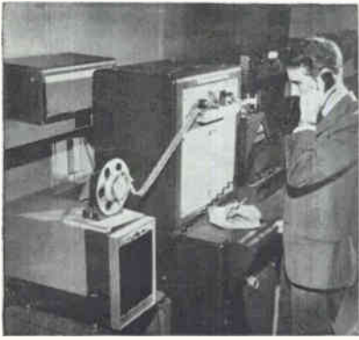
ENGINEERING changes are transmitted by Martin Co. to missile base using Digitronics' Dial-o-verter terminal
