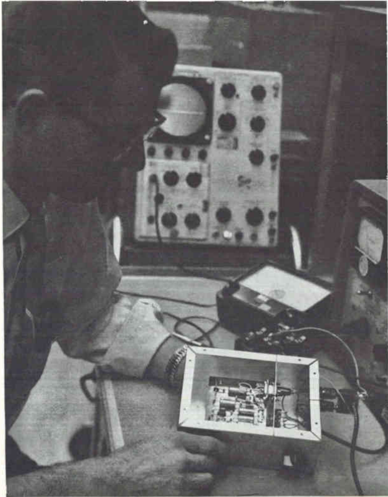
AUTHOR FLEENOR checks performance of low-noise field-effect transistor preamplifier
