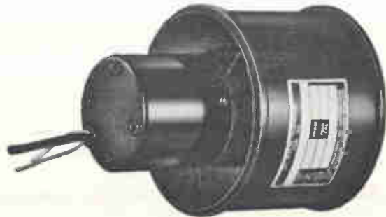
A 3" blower may operate more than 10,000 hours on d.c. using an inverter that adds 1½" to motor length.
