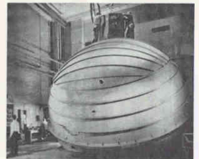
BUTTONED-UP CHAMBER. Men at top adjust solar simulator, while those at left control simulated space phenomena
