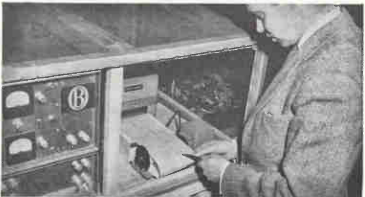
The Honeywell Model 906 Visicorder Oscillograph—with a Honeywell Model 119 Amplifier—record circuit bushing tests for Ohio Brass.
