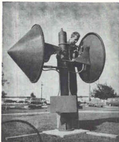
BISTATIC doppler radar installed by Sylvania at Nike Hercules missile base detects person stepping inside electromagnetic field
