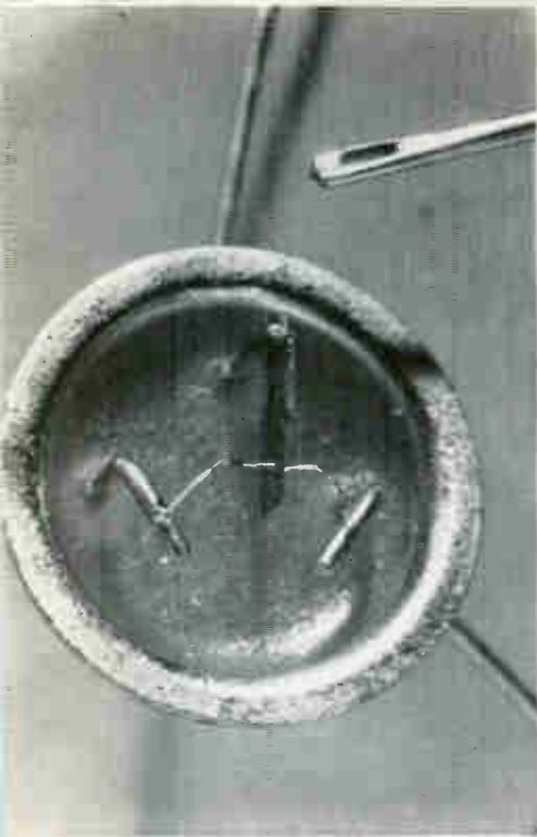
FINE CONTROL possible with lasers is demonstrated by welding of transistor lead wires to header. Hughes laser makes weld in less than 1 msec
