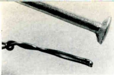
LASER WELD of 0.004-in.-diameter copper-constantan thermocouple. Hughes says wires need not be stripped
