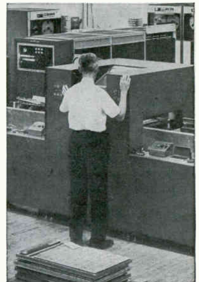
OVERALL checking equipment includes handler unit (in front of operator), data processor and core memory (behind handler unit), tape drives and typewriter
