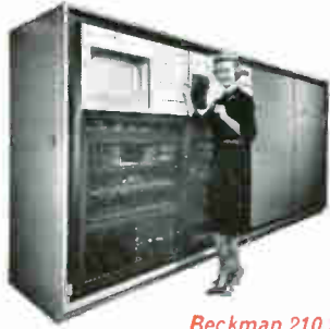
Beckman 210 high-speed, solid-state, data processing system shown with cathode ray oscilloscope monitor.
