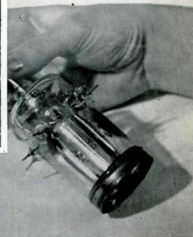
PERFORMING laser mode-separation measurement with transmission-type microwave phototube. Large photo shows phototube withdrawn from its traveling-wave-like focusing structure
