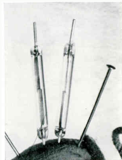
SMALL reed switch is only 0.1-in. in diameter, each has switch arms of equal length (General Electric)
