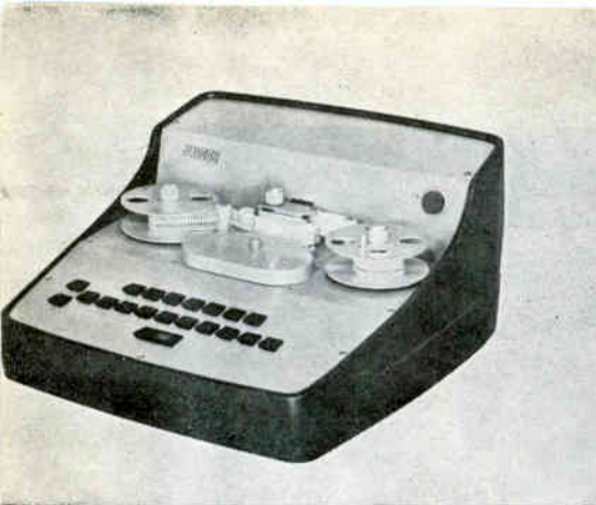
VISUAL PRINTOUT , magnetic keyboard, remote programming ability feature Navigation Computer's tape-puncher for numerical machine control
