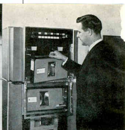
CARTRIDGE-LOADING tape-drive system introduced by IBM has an instantaneous data rate of 170,000 8-bit characters a second
