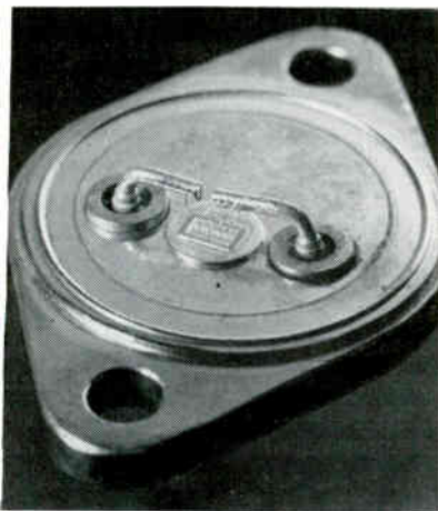
HIGH-FREQUENCY power transistor has mesa configuration and makes use of interdigitated emitter and base fingers to increase junction area
