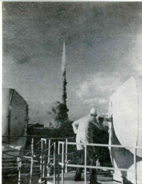
NIKE ZEUS in test firing is framed by two missile-track radars that will guide it to the intercept point
