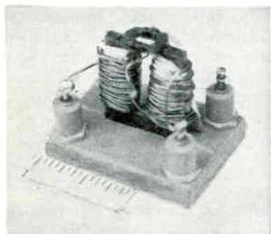
INDUCTOR L_1 for sweep-frequency oscillator
