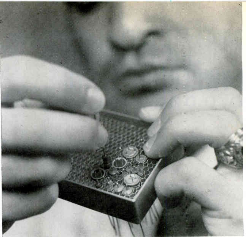
ALUMINUM cell material in honeycomb matrix is flexible enough to permit insertion of various sized components
