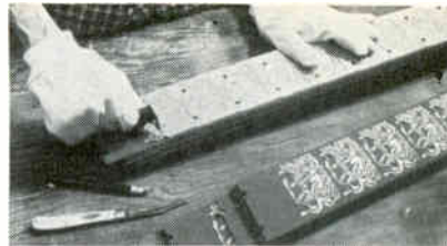
SCRAP COPPER is easily peeled from stamped phenolic strips
