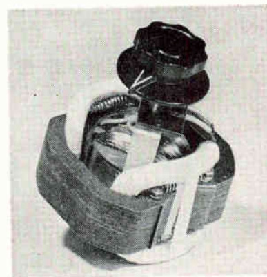
S.E.I.M. brushless transformer varies output by changing angle of secondary winding
