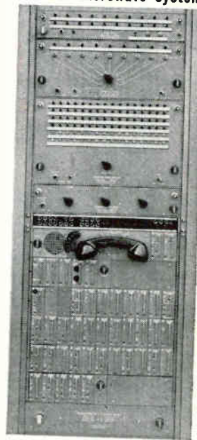
Typical master station used by Western Union on their MLD-4B Transcontinental Microwave System.
