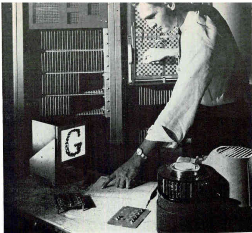
FIG. 6—Testing Aeronutronic general-purpose learning system with alphabetic character input. System uses 200 Mind components
