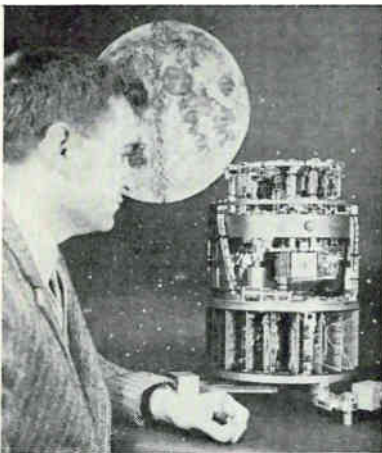
SURVEYOR moon probe, to be launched next year, will carry this lunar seismometer built by ITT Federal Labs and designed by Lamont Geological Observatory
