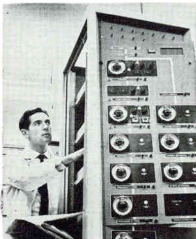
Console, by Stromberg-Carlson, displays Project Mercury capsule flight data and astronaut's reactions
