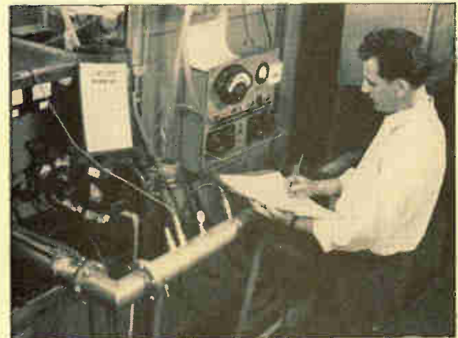
Life testing of Raytheon tubes, such as the QK-358 magnetron, for six weeks or more serves as a quality check of their performance characteristics as recorded and plotted against time.
