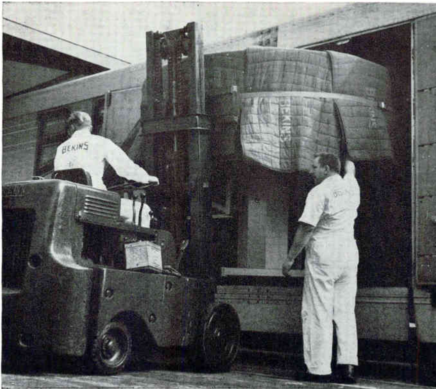
Loading a Genisco Model A 1030 G-Accelerator into one of Bekins Electronics Vans. Unit measures 106 inches wide by 137 inches deep. Weight uncrated is approximately 2000 lbs.
