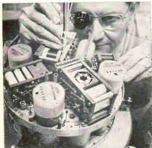
REPEATER is built to operate for 20 years under 2½ miles of sea water (photo above)
