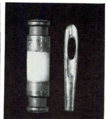
Heart of amplifier—a hermetically sealed gallium arsenide diode—is compared with eye of average-sized sewing needle.
