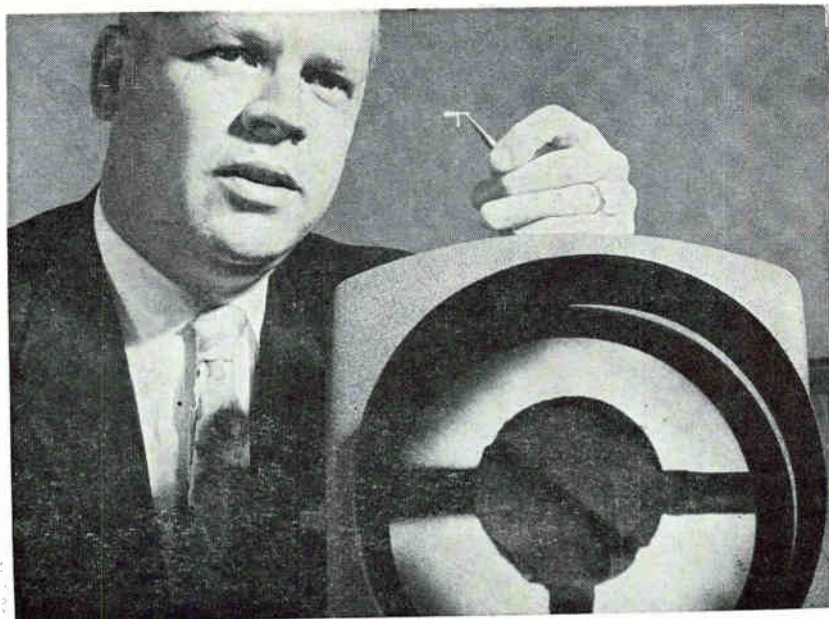
BASE AND EMITTER plates are visible in comparator scope. Inventory control of transistors is improved because of flexibility in adding cases of various types after basic transistor unit is completed
