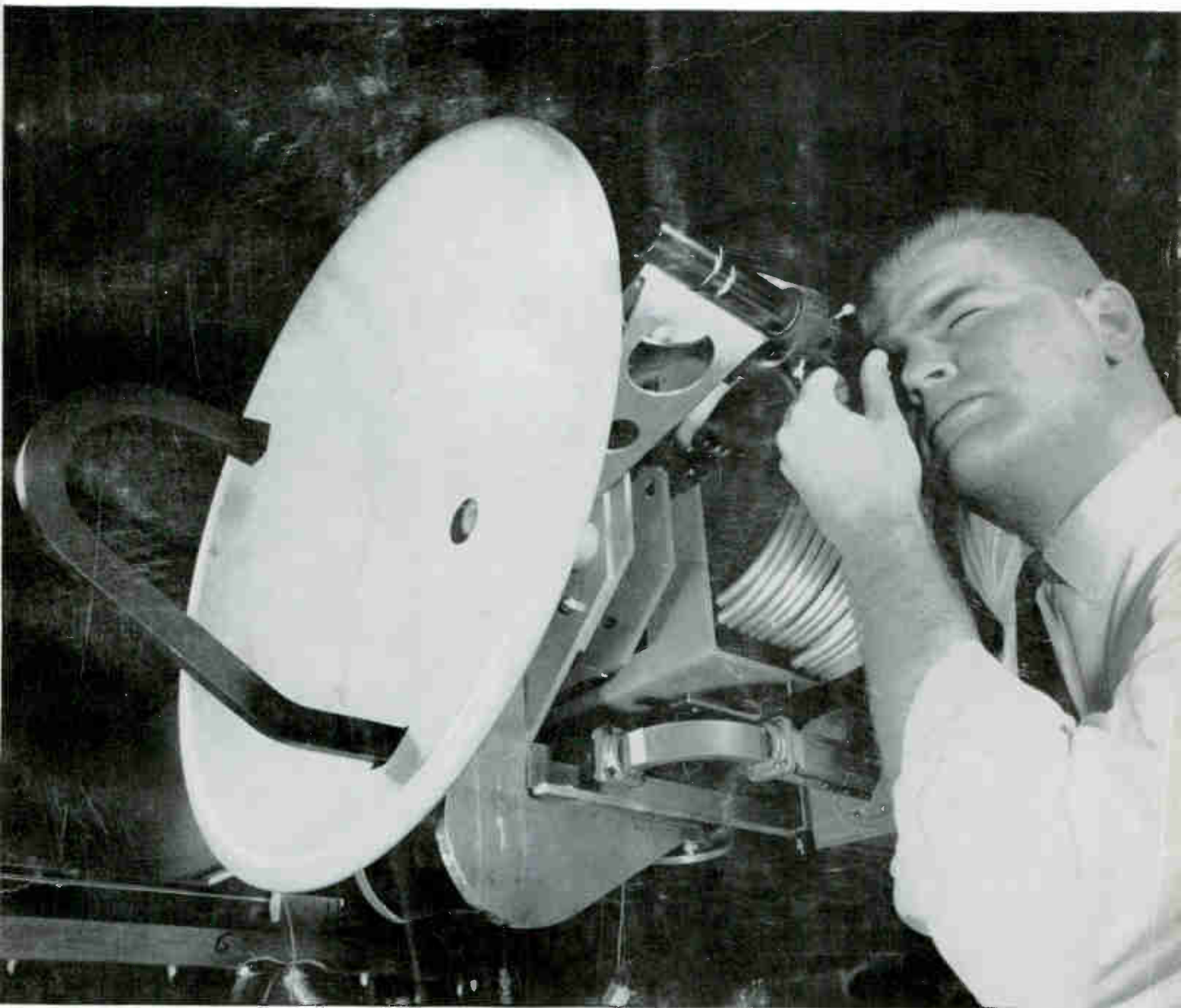
BORESIGHTING antenna for radar cross-section measurements. But how good will they be?
