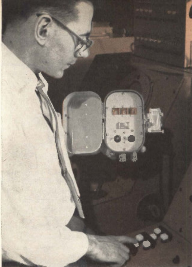
REMOTE COMMUNICATOR UNIT enables checkout system to "converse" with operator of system. By code numbers, checkout system instructs operator to change switch positions, and compare displays. Operator replies by pressing YES and NO buttons—Fig. 11
