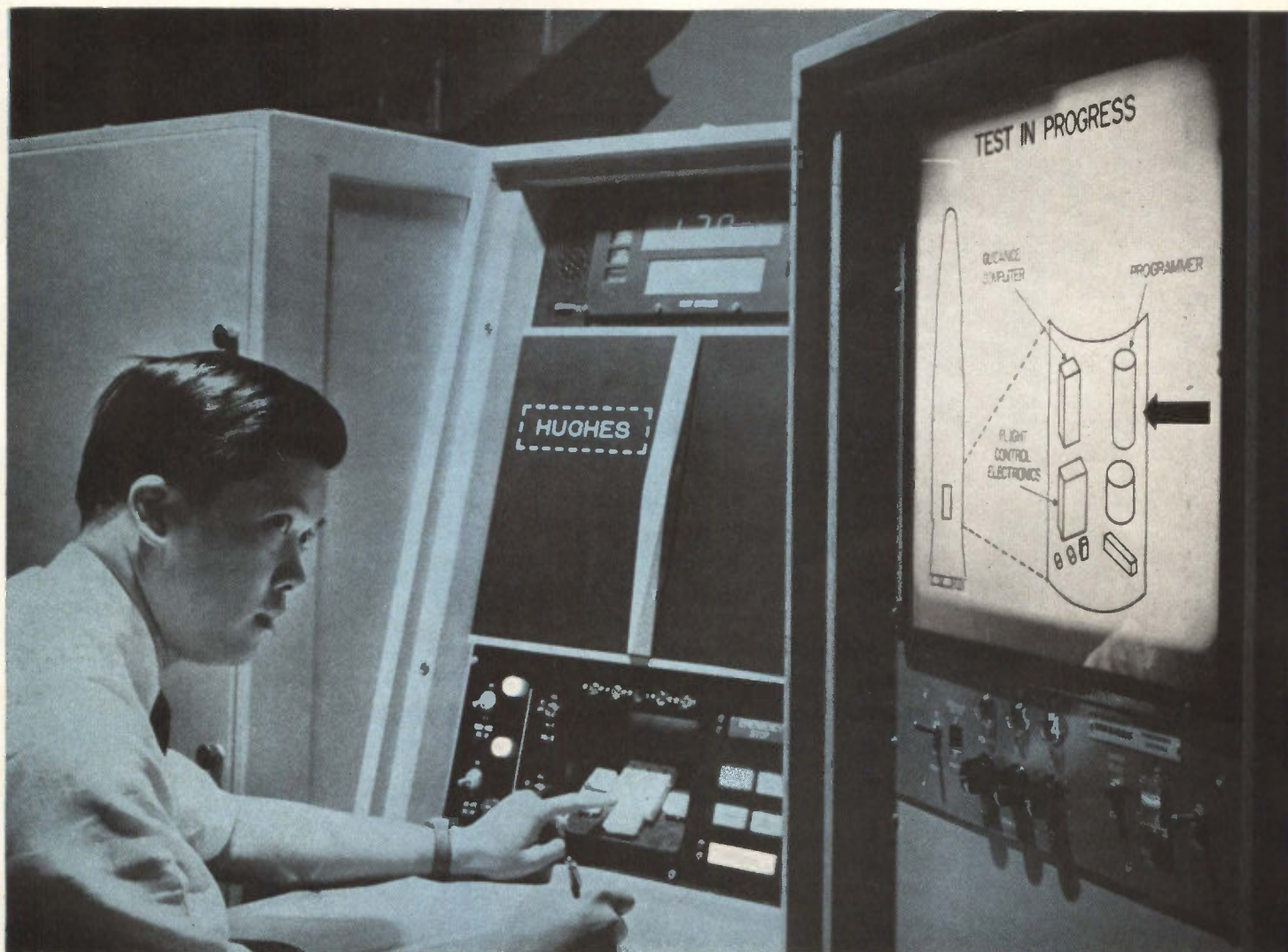
AUTOMATIC ELECTRONIC ANALYZER D-PAT (Drum-programmed Automatic Tester) by Hughes Aircraft uses digital computer control to test ICBMs and predict operation. System flashes large-screen picture of missile electronics with arrow indicating malfunctioning component
