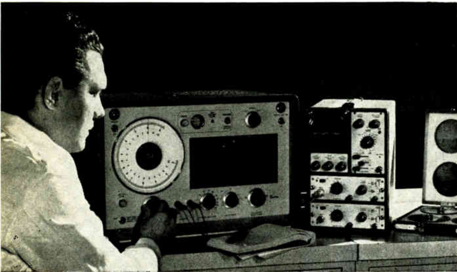
FIG. 1—Function generator disk can be rotated in both directions, as indicated by the cps scale
