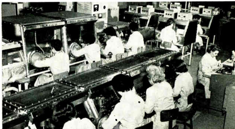
Transistor manufacturing line has stations for washing, rinsing, vacuum bakeout, filling, sealing, welding. Arm rests and built-in lighting are aids to production
