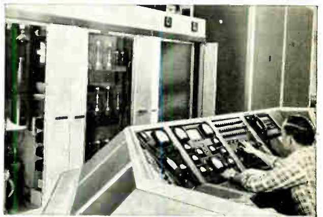
Partial view of the transmitter, console and control panel for the radar system.
