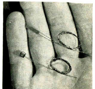
Transverse field Hall device (top), and axial field sensor (bottom)
