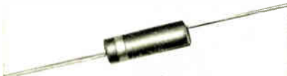
Type 8292ZN* (Bulletin 131B6) Metallized Paper Plastic Cased Tubular -30°C to 100°C 200, 400, 600 DCWV .01 to 2.0 mfd 1 4" x 19 32" to 1" x 2-3/8"
