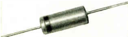
Type V146X*-V146XR* (Bulletin 142B2) Mylar "Wrap and Fill" Flat and Round Styles -65°C to 85°C 150, 200, 400, 600 DCWV .001 to 2.0 mfd .156" x 1 2" to 1.421" x 3"
