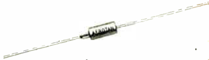
Aerotan® Types ST12*-ST13* (Bulletin 215B2) Solid Tantalum Electrolytic Metal Cased Tubular -80°C to 125°C 6 to 35 DCWV 1.0 to 330 mfd .125" x .250" to .341" x .750"
