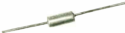
Type 83Z* (Bulletin 131B2) Metallized Paper Thermoplastic Cased Tubular -15°C to 85°C 200, 400, 600 DCWV .0005 to .04 mfd 3 16" x 7/16" to 1/4" x 9/16"
