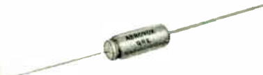
Types CRE-QRE* (Bulletins 201B6 & 201B7) Aluminum Electrolytic Metal Cased Tubular -40°C to 85°C 3 to 150 DCWV 1 to 500 mfd 3 16" x 1 2" to 3 8" x 1-1 2"
