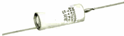
Type SRE* (Bulletin 201B1) Aluminum Electrolytic Metal Case Tubular -0°C to 65°C 3 to 150 DCWV 1 to 500 mfd 3 8" x 1" to 1/2" x 1-5/8"
