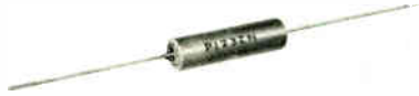
Types P123ZN-323ZN* (Bulletin 131B8) Metallized Paper Metal Cased Tubular -55°C to 125°C 50, 150, 200, 400, 600 DCWV .001 to 12.0 mfd .175" x 7/16" to 1" x 2-9/16"
