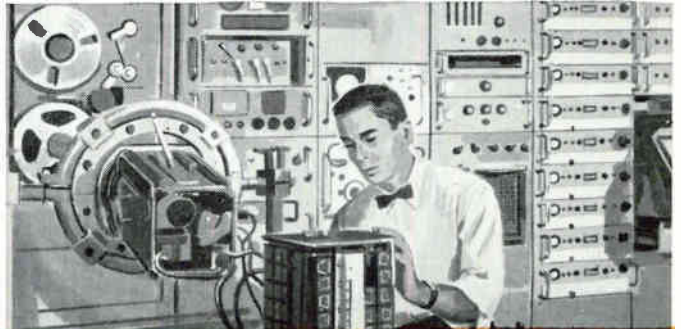
GAC telemetry system tester checks out airborne telemetry package for Navy's SUBROC missile.
