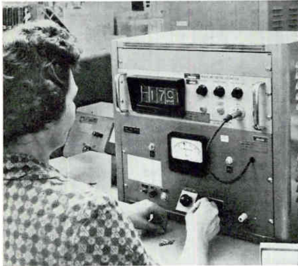
QUALITY CONTROL OF ELECTRONIC COMPONENTS. More than 50 NLS 481 digital voltmeters are used in the Quality Assurance Program at the Semiconductor-Components Division of Texas Instruments Incorporated. The instrument pictured is measuring breakdown voltages of high-reliability germanium switching devices.
