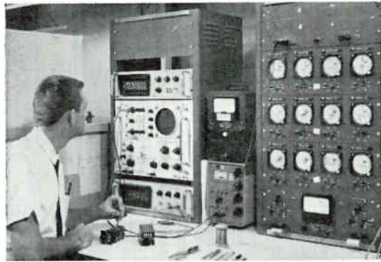
MISSILE CHECKOUT. Two NLS DVMs team up on checkout of equipment for the GAM-77 Hound Dog Missile at the West Coast Laboratories of Mallory Electronics Company, A Division of P. R. Mallory & Co. Inc. The 481 (bottom) calibrates remotely settable timers for the Hound Dog and the V35 (top) is used for final checkout of these devices. "By using DVMs, we are able to eliminate human error in final inspection," said a Mallory executive.
