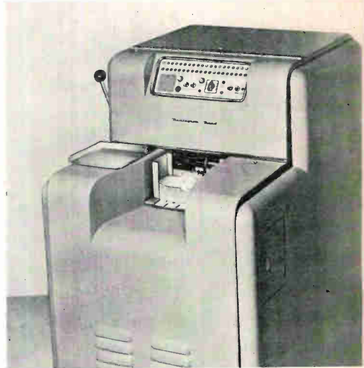
With this optical scanning punch, 40 field markings on each side of a special 90-column card can be read at the rate of 150 cards a minute
