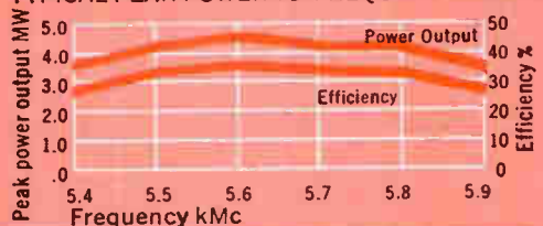
TYPICAL PEAK POWER VS. FREQUENCY-130KV
