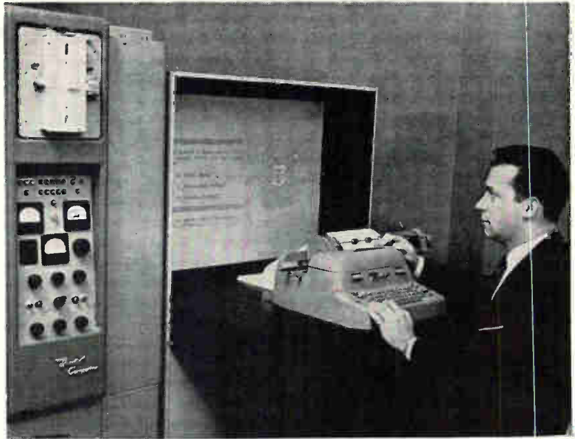
Computer (left) and screen of random-access projector (right) are key elements in SDC teaching machine
