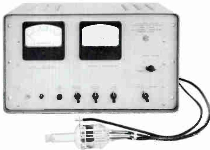
Pressures from 10^{-3} to less than 10^{-10} Torr are measured with high stability and linearity by Model 751 Nottingham Gauge Control, which will operate any commercial Bayard-Alpert type ionization gauge.
