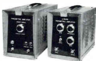
Parametric Amplifier with regulated power supply developed for use in 700 to 3000 mc range.
