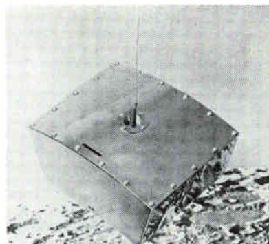
Satellite is a foot square and a half-foot deep
