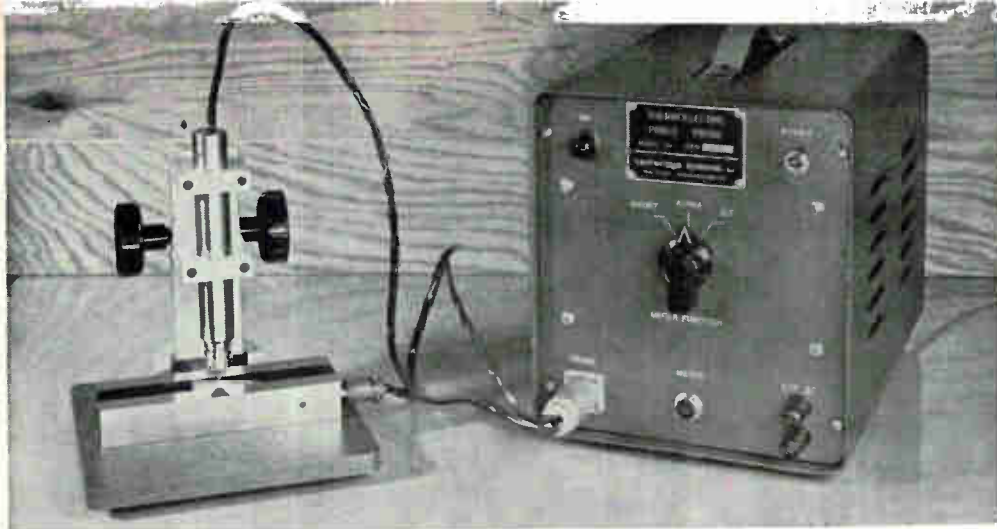
Point of the heated vertical probe is applied to the sample between lower clamps. Control on right monitors probe temperature through thermistors, also feeds thermoelectric voltage to an external differential meter that indicates junction polarity
