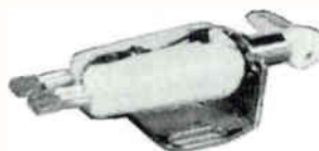
STEREO CARTRIDGE Crystal—"PIEZO" Y-130 X'TAL STEREO CARTRIDGE At 20^{\circ}\text{C} , response: 50 to 10,000 c/s with a separation of 16.5db. 0.6V output at 50 mm/sec. Track- ing force: 6 \pm 1\text{gm} . Compliance: 1.5 \times 10^{-6} cm/dyne. Termination: 1M \Omega + 150pF.
