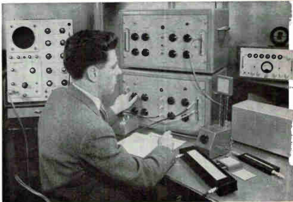
Operator prepares to display pulse waveforms on the small square screen
