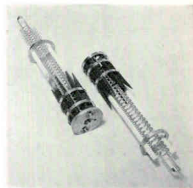
Meanderline traveling wave tube gets its name from shape of tubes used to conduct signal
