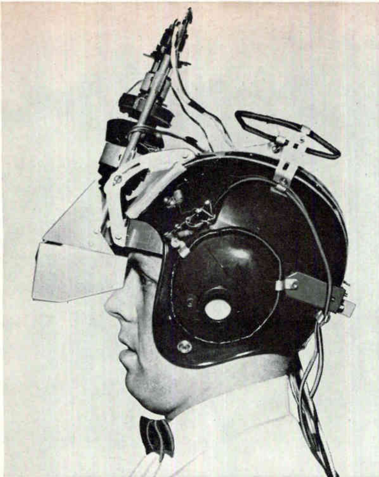
FIG. 2—Author Comeau demonstrates experimental model of the headsight viewer
