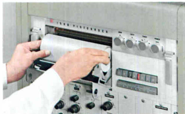
The loading of recording paper into the 1508 is a simple process. The roll of paper drops easily into the receptacle with no need for threading.
